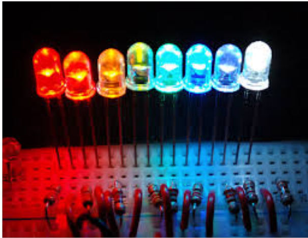
LED (Light-Emitting Diode)
